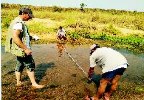
Water depth and velocity measurement (a) in river Kathajodi (Mahanadi delta) for e-flows simulation study (b)-HEC-RAS model
